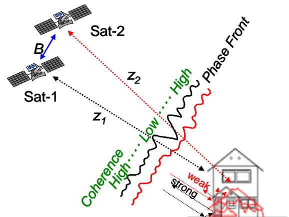
Fig.1 Schematic diagram for detecting building damage using repeat-pass radar observations
