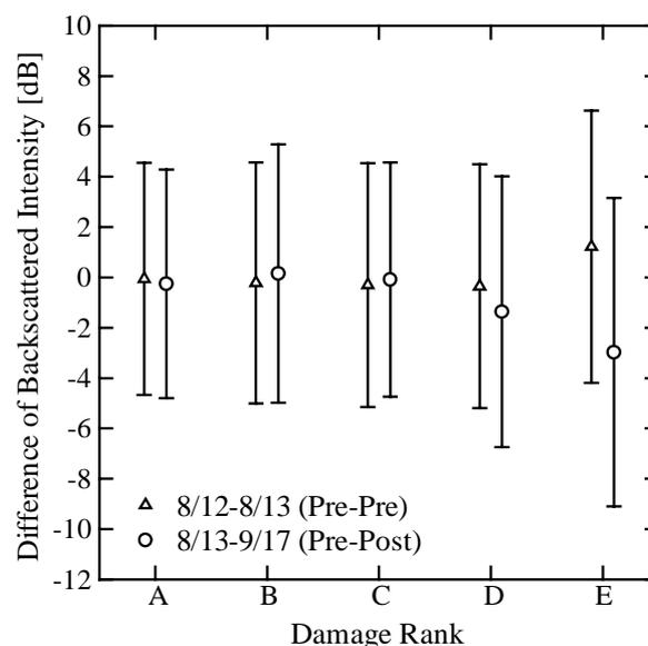
Fig. 7 Difference in backscattered intensities from two time instants for different damage rank
