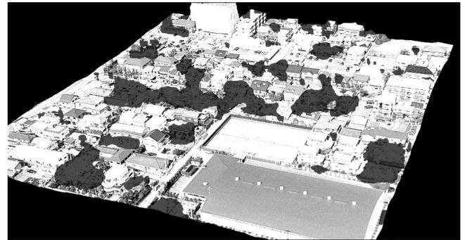
Fig. 7 Damaged buildings extracted by texture analysis
