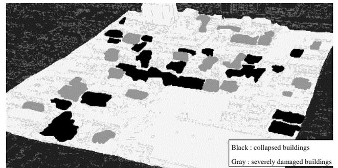
Fig. 8 Damaged/collapsed buildings by ground survey and visual inspection of HDTV images
