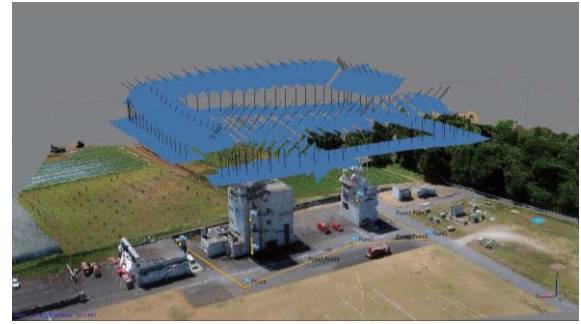
Fig.3 Developed 3D model and estimated camera position by SfM
