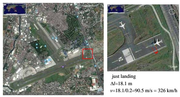
**Figure 1** Pansharpened QuickBird Image of Ninoy Aquino International Airport, Manila, Philippines, from Google Earth. A ghost is generated in front of the just landing airplane.
