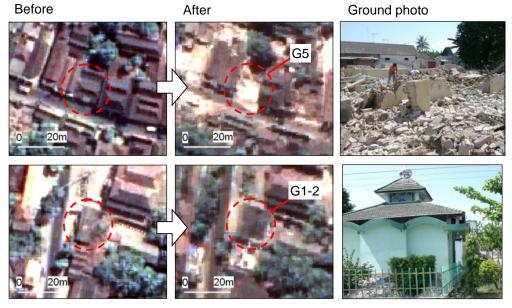
Fig. 5 Comparison of pre- and post-earthquake QB images with ground photographs
