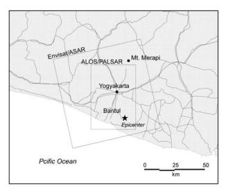
**Figure 1.** The area subject to analysis for the 2006 Mid Java, Indonesia earthquake. The areas inside the rectangle indicate the region of interest in ALOS/PALSAR and Envisat/ASAR, respectively.
