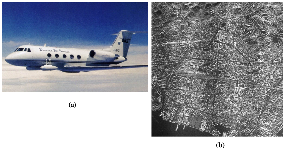
Figure 6: Aircraft equipped with SAR system (a); and image of Nagata area, Kobe (b) [CRL and NASDA, 1998]
