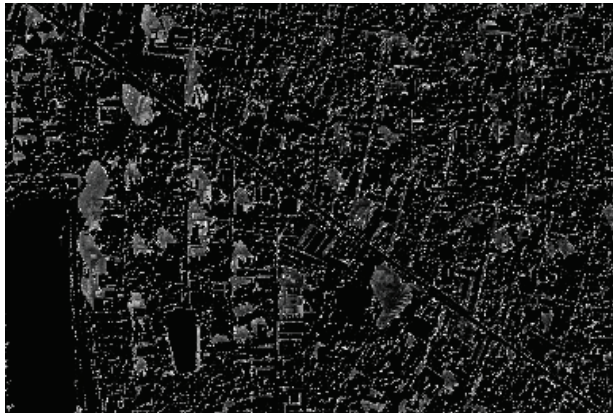
Fig. 6 Extracted pixels (gray and white) as in shadow.
