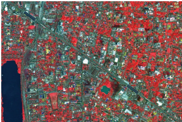
Fig. 11 False color composite for the shadow-corrected QuickBird Image
