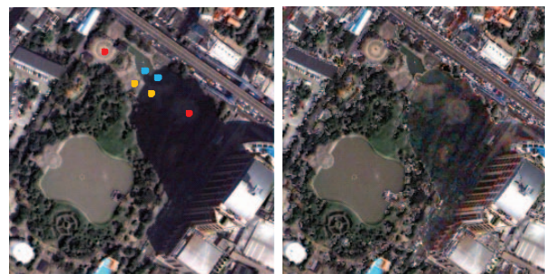
Fig. 8 True color composite of the original image (left) and the shadow-corrected image (right) for area A
