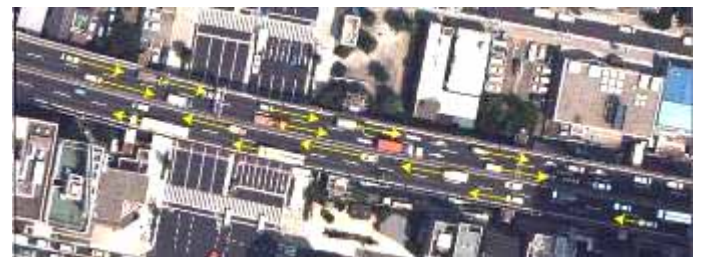
Figure 14. Result of automated speed detection from two consecutive aerial images of Roppongi.
