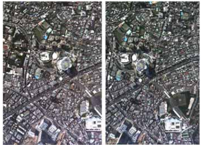
Figure 4. Two consecutive digital aerial images of Roppongi, Tokyo, with about 80% overlap.
