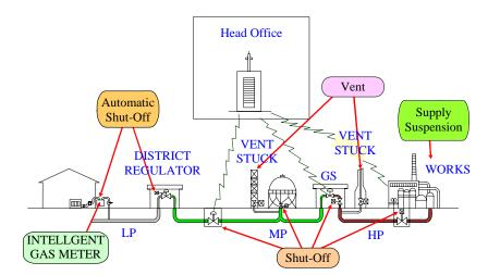
Figure 1. Outline of emergency control of natural gas supply system in Japan
