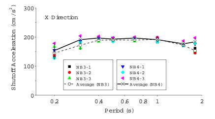
Figure 4. Shutoff accelerations with respect to the periods of sinusoidal waves applied to the X direction
