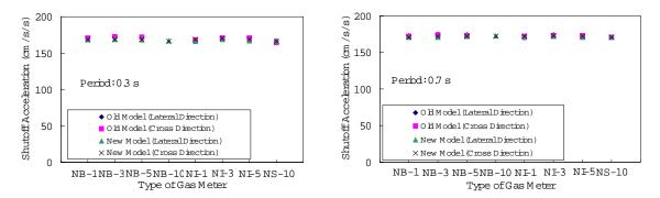
Figure 2. Shutoff acceleration of various types of intelligent gas meters conducted by producteers (Old model: until February 2003, New model: from February 2003)
