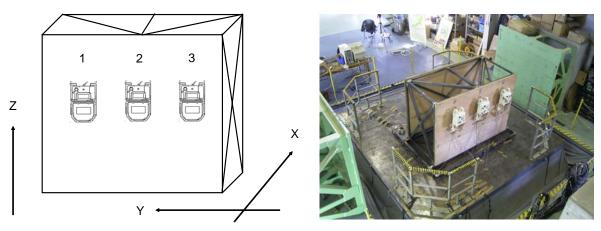
Figure 3. Shaking table test of intelligent gas meters
