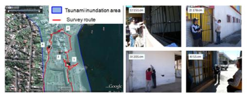
Fig. 10: Measurement of tsunami inundation depth in Talcahuano
