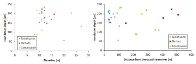
Fig. 11: Summary of the measurement of tsunami inundation depth
