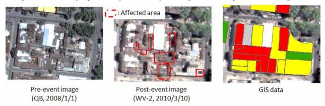
Fig. 7: Comparison between pre- and post-event satellite images to detect affected buildings field photos to show the examples of damaged buildings.
