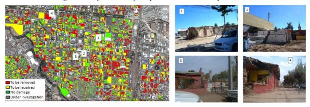
Fig. 5: GIS file to show the damage levels of buildings in Talca and locations of field photos
