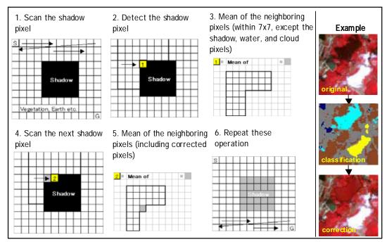
Figure 6. The flow of the correction of the shadow areas and the example of the correction.
