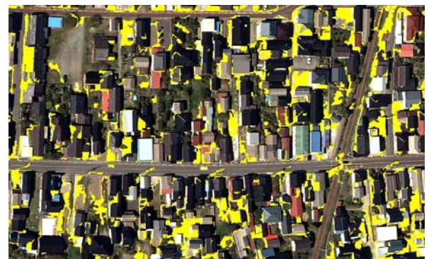
Figure 11. The result obtained by applying the debris extraction procedure to the pre-event digital image.
