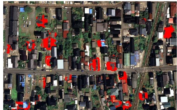
Figure 3. The result of visual extraction of debris.
