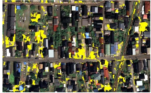
Figure 10. The result of extracted debris by the object-based level-slice method. Many small commission errors are seen.
