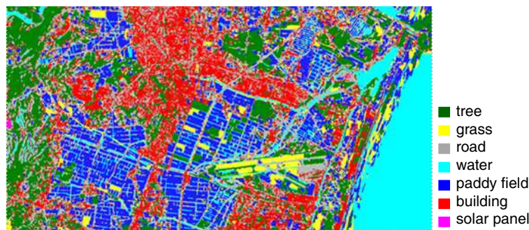
Figure 9. Supervised land-cover classification result for the first two PC images of the original full-polarizations plus first five PC images of their texture measures.
