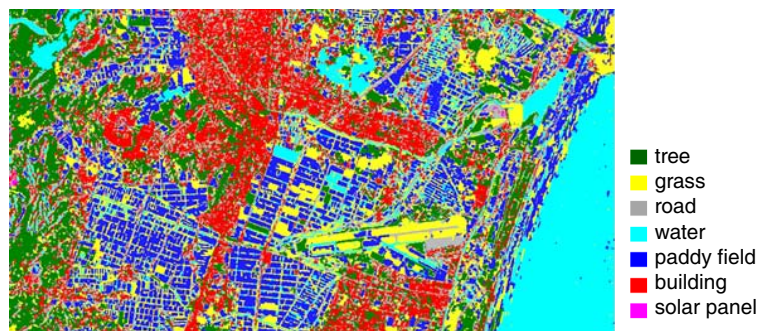
Figure 7. Supervised land-cover classification result for the original HH and HV polarization images.
