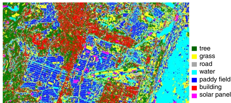
Figure 7. Supervised land-cover classification result for the original HH and HV polarization images.
