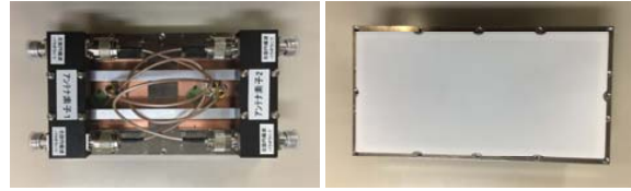
(a) Two microstrip antenna (b) Radome of feeder Fig.9. Microstrip CP antenna as feeder of parabolic antenna
