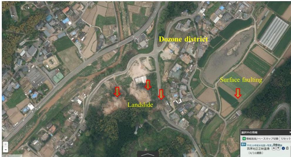
**Figure 11. Orthorectified photo taken on April 16 by GSI over Dozone district. The surface faulting shown in Figure 2 and several landslides can be recognized.**
