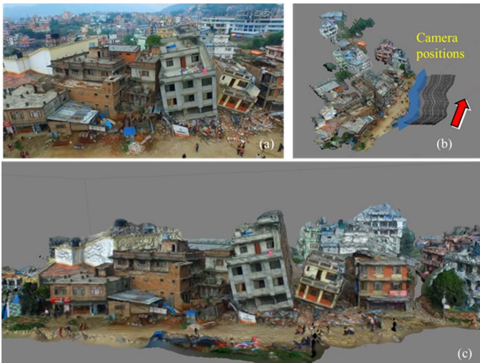
Figure 9 A snapshot of video footage over Sitapaila in Kathmandu (a), estimated camera positions by SfM (b) and developed 3D model of the district (c).
