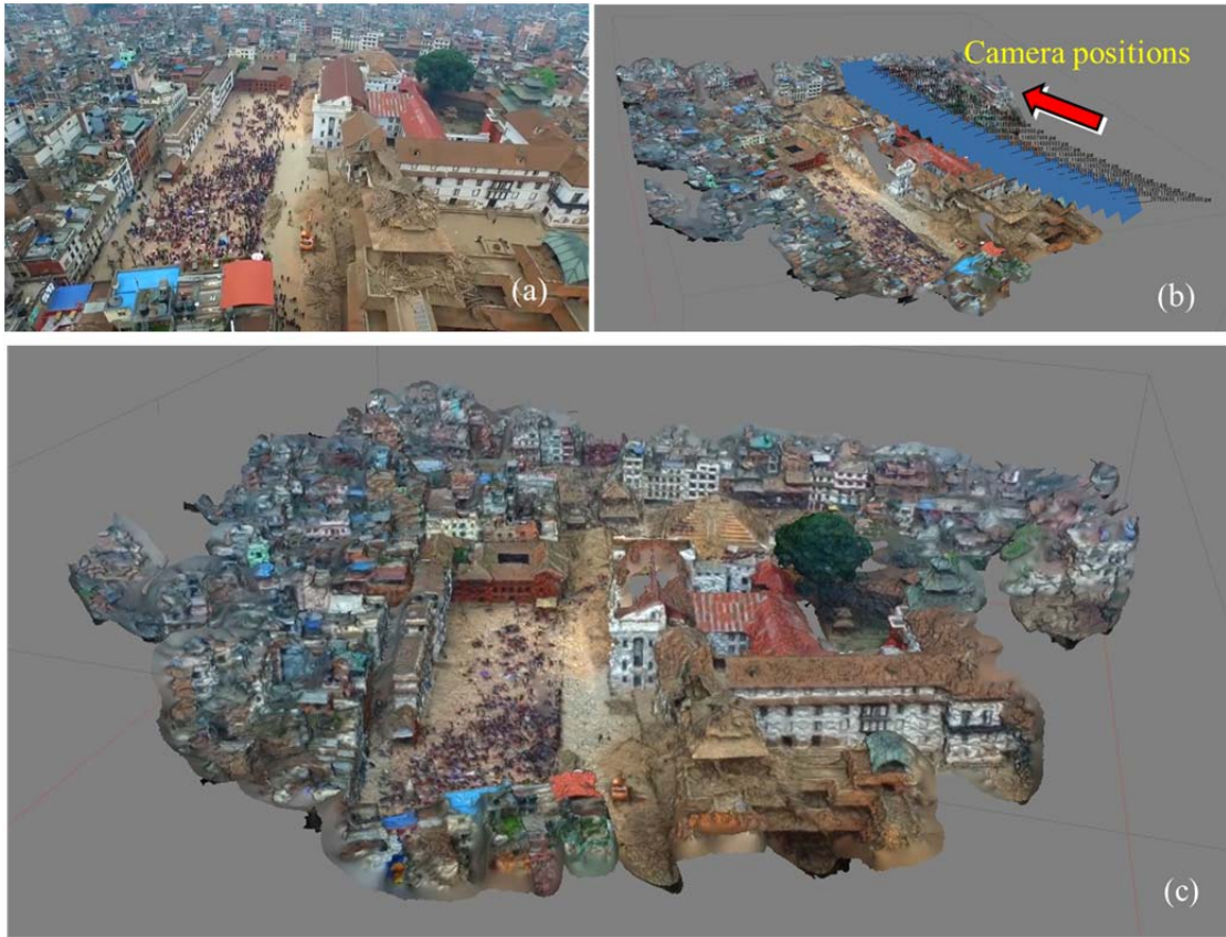
Figure 8 A snapshot of video footage over Durbar Square in Kathmandu (a), estimated camera positions by SfM (b) and developed 3D model of the district (c).
