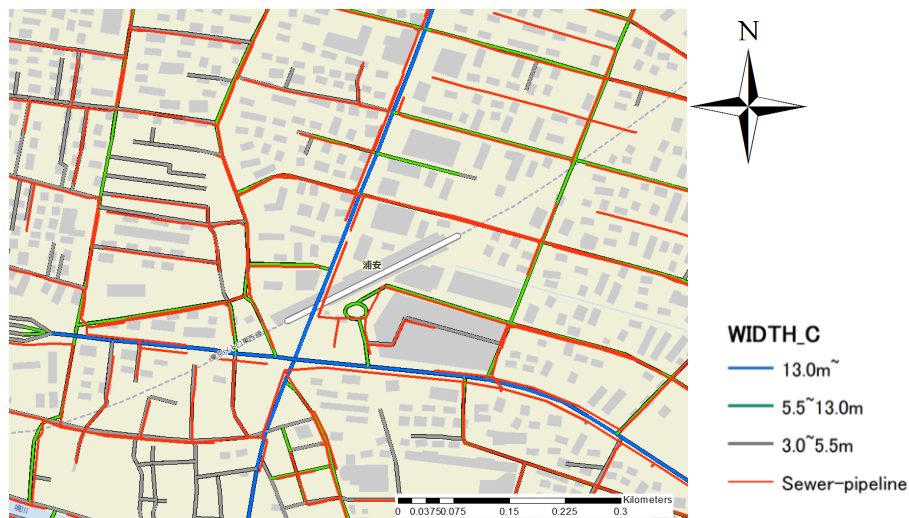
Figure 7. Roads and sewer pipelines around the Urayasu subway station
