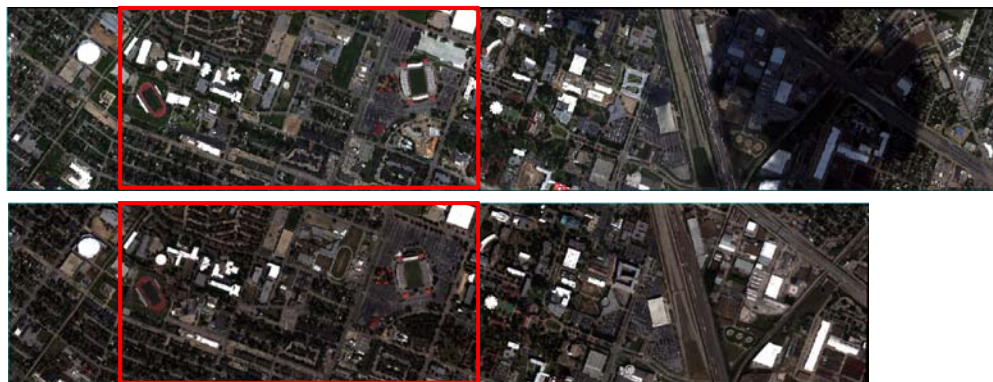
Figure 2. True color composites of the hyperspectral image (top) and the multispectral image (bottom) for the CASI-1500 imaging area. The red square shows the study area.
