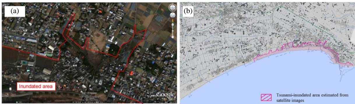
Figure 4: (a) Example of visual inspection of satellite images to identify tsunami-inundated areas and (b) their visualization in GIS system
