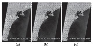
Figure 5 Detected displacement vectors in each sub-area in the periods: Oct. 21, 2010 to March 13 (a), to March 24 (b) and to April 4, 2011 (c), overlapping on the color composite of the TSX intensity images.
