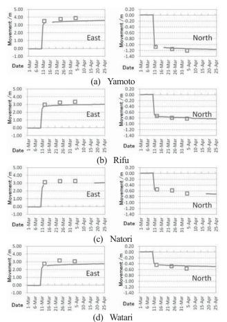
Figure 8 Comparison of movements converted from GPS data at Yamoto (a), Rifu (b), Natori (c), and Watari (d) ground control stations and the results detected in surrounding 13 km<sup>2</sup> sub-areas.
