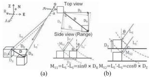
Figure 7 Schematic views of the horizontal (a) and vertical displacements (b) in a SAR image.
