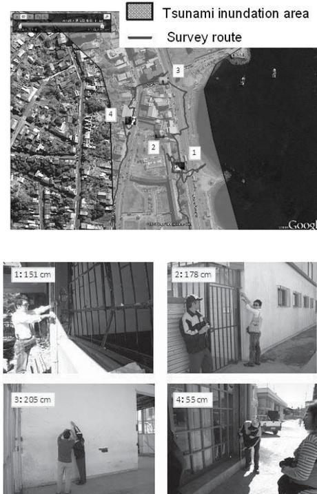
Figure 10 Measurement of tsunami inundation depth in Talcahuano
