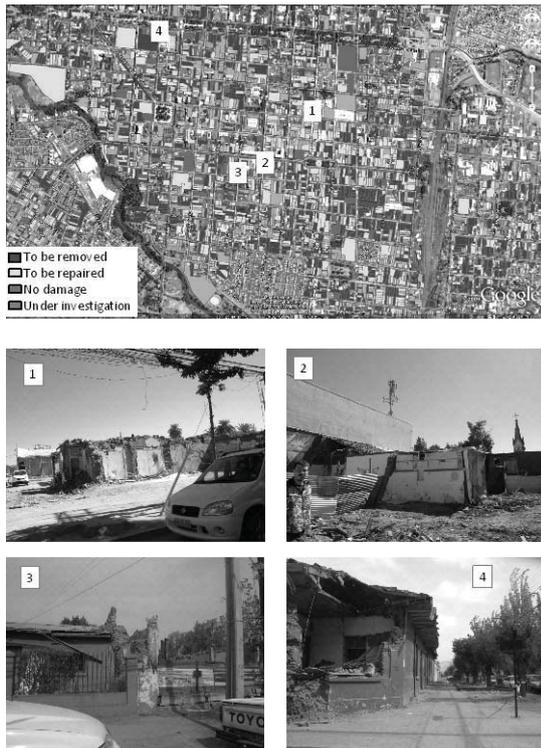
Figure 5 GIS file to show the damage levels of buildings in Talca and locations of field photos
