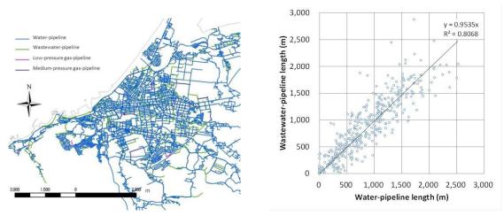
Figure.7. Various pipeline data on GIS in Kashiwazaki. Figure.8. Relationship between water pipeline and wastewater line length in 250m grid in Kashiwazaki.
