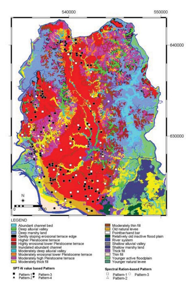
Figure 2: Geomorphological map with Landfills. Both the patterns derived from SPT-N values of boreholes and spectral-ratios of microtremors were superimposed in this map.
