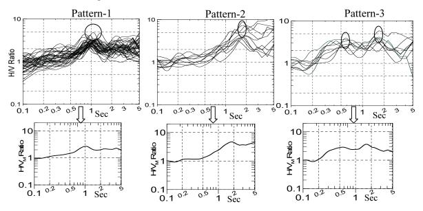
Figure 9: Spectral ratio curves and their normalized average shape as obtained from the analyses microtremors records on nine geomorphic units.
