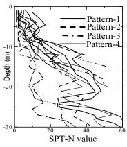
Figure 7: SPT-N value curves of four different patterns
