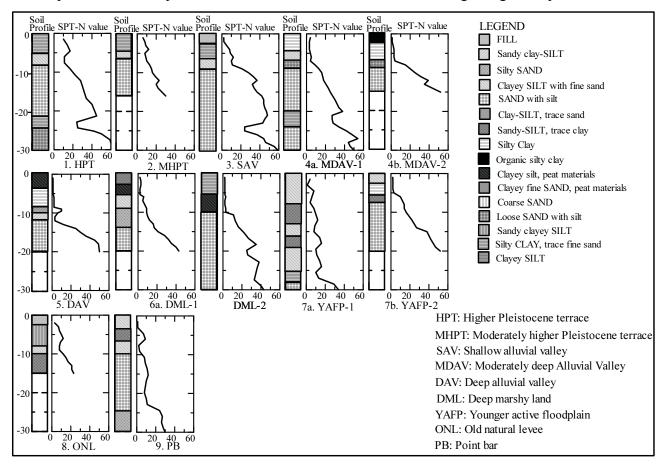
Figure 4: The representative soil profiles and SPT-N value of boreholes
