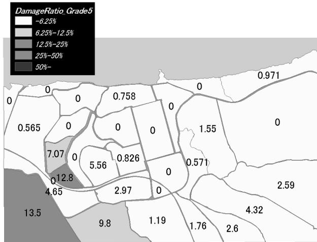
**Figure 7. Building damage ratio (number of Grade-5 buildings in each block divided by the total number of buildings in each block) of Boumerdes city by visual interpretation using QuickBird images (Kouchi et al., 2004)**
