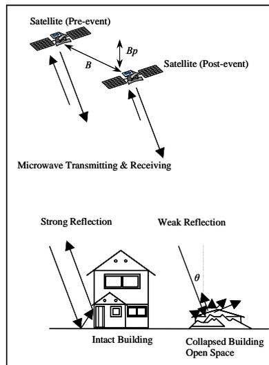
**Figure 5. Schematic figure of the geometry of repeat-pass satellite observation and backscattering characteristics of objects on the earth’s surface**
