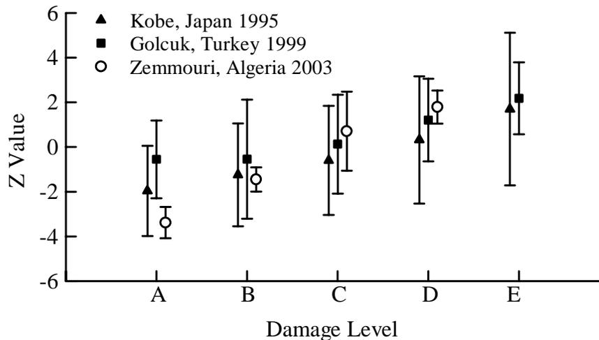
**Figure 10. Relationship between  $z$  value and damage level for SAR images from the three earthquakes**
