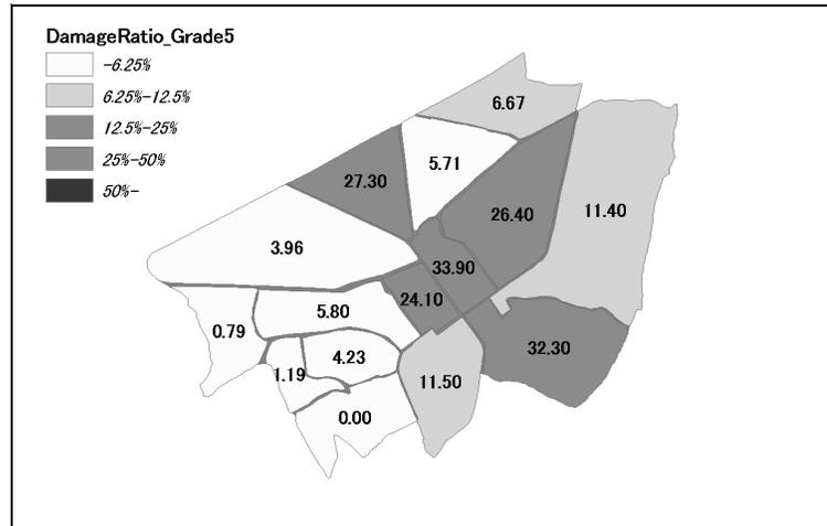
**Figure 9. Building damage ratio (number of Grade-5 buildings in each block divided by the total number of buildings in each block) of Zemmouri city by visual interpretation using QuickBird images (Kouchi et al., 2004)**
