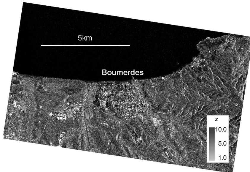
**Figure 6. Distribution of the value  $z$  overlaid on the intensity image taken over Boumerdes city using RADARSAT satellite**
