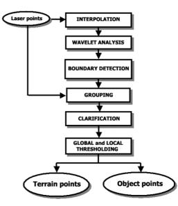
Figure 1. The components of the processing system
