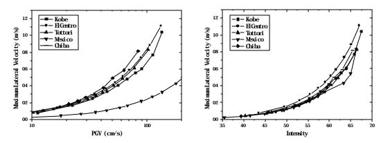
Figure 6. Relationship between the maximum lateral velocity of the vehicle and the peak ground velocity applied to the transverse direction to the vehicle (left) and the relationship between the maximum lateral velocity of the vehicle and JMA intensity (right)
