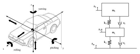
Figure 1. Fundamental motions of a vehicle
