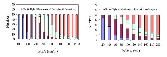
Figure 1. Number of occurrence of each damage rank in different excitation levels.
