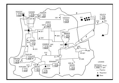
Figure 9. Distribution of SI and PGA in Taipei Observed by New SI Senors in the 1999 Chi-Chi Earthquake
