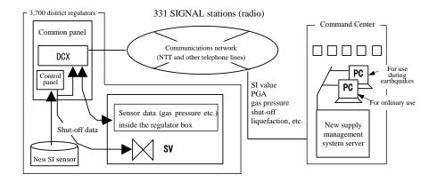
Figure 7. System Configuration of SUPREME
