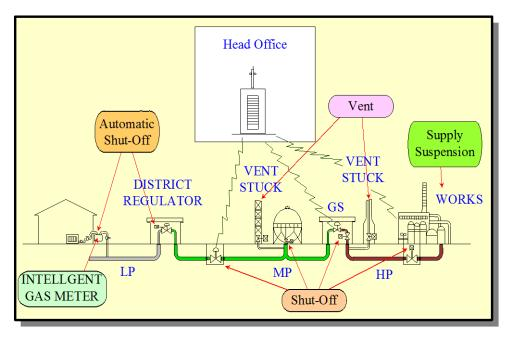
Figure 2. Emergency Shutoff Systems of Natural Gas Network of Tokyo Gas Co., Ltd.
