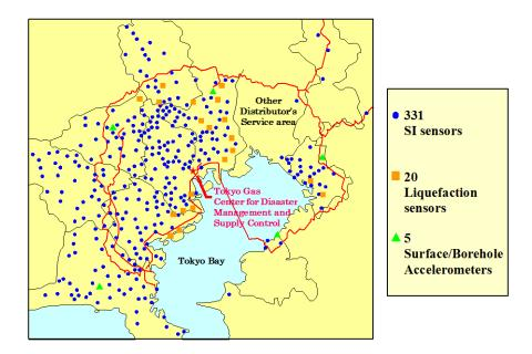
Figure 4. Seismic Monitoring Sensors of SIGNAL
