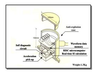
Figure 5. New SI Sensor
