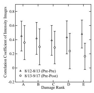
Fig. 8 Correlation coefficient of intensity images between two time instants for different damage rank
