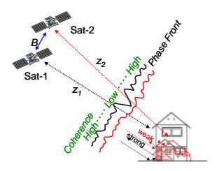
Fig. 1 Schematic diagram for detecting building damage using repeat-pass radar observations
