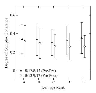
Fig. 9 Degree of complex coherence between two time instants for different damage rank
