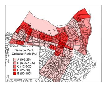
Fig. 3 Distribution of building collapse ratio in Golcuk by the field survey of AIJ
