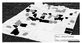
Fig. 8 Damaged/collapsed buildings by ground survey and visual inspection of HDTV images
