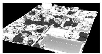
Fig. 7 Damaged buildings extracted by texture analysis
