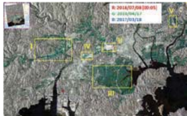
Fig. 1 Color composite of three-temporal PALSAR-2 images for Kurashiki and Okayama City area
