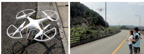
Fig. 2 Phantom 3 Professional UAV used in this study (left) and a scene of manual operation flight (right)
