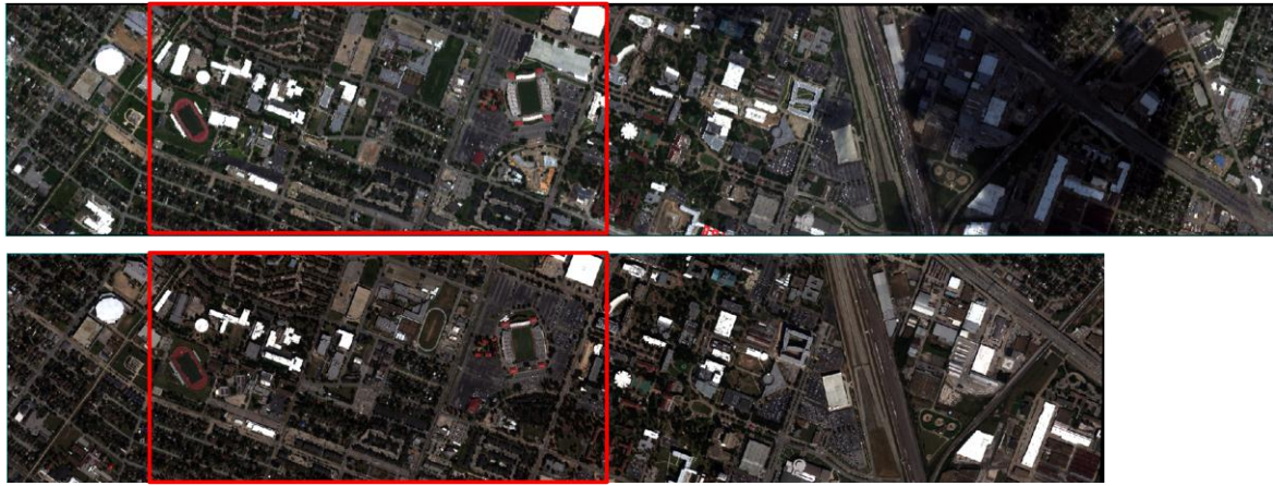
Fig.2 True color composites of the hyperspectral image (top) and the multispectral image (bottom) for the CASI-1500 imaging area. The red square shows the study area.
