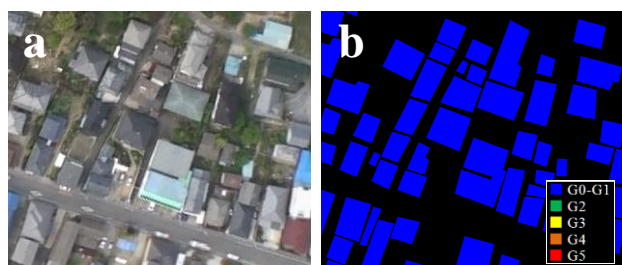
Fig.4 a: Aerial visible image of non-damaged area, b: Damage classification in the same area.
