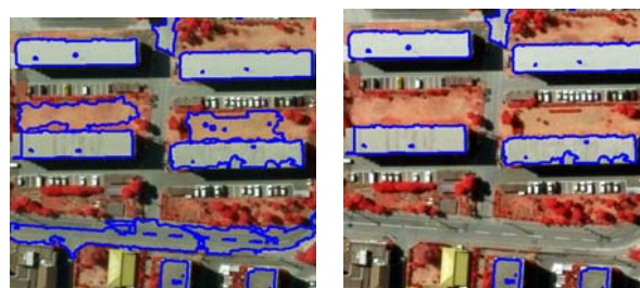
Fig.8. Comparison between before and after the Building Detection Corrections using Shadows (a) Before Correction, (b) After Correction
