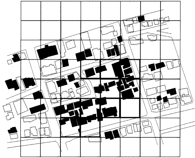
Figure 6. Size of pixels in ERS image compared to actual buildings and city blocks. Thick black grid indicates the pixels representing the areas with the severe damage ratio equals to 100%.
