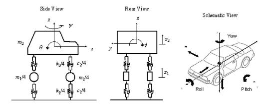
Figure 4. Vehicle model with six-degrees-of-freedom used in this study.
