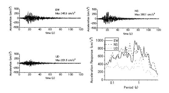
Figure 3. Acceleration time histories recorded at K-NET Taiki during the 2003 Tokachi-oki earthquake and their acceleration response spectra with 5% damping ratio.
