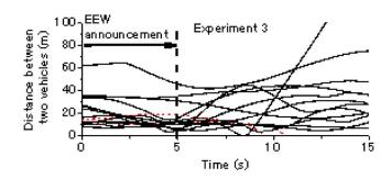
Figure 13. Distance between the two vehicles in Experiment 3. Two traffic accidents were caused and those results are shown by dashed lines.
