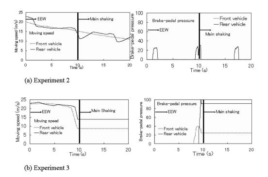
**Figure 14.** Example of time histories of moving speed and brake-pedal pressure in (a) Experiments 2 and (b) 3. The example of Experiment 3 shows the result of the collision from behind.
