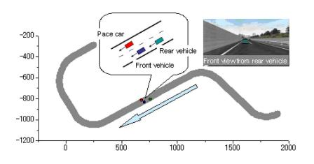
**Figure 2.** Scenario expressway course in the experiment. The three vehicles can see one another through windows and mirrors.
