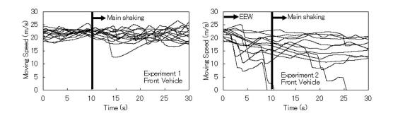
Figure 11. Comparison of moving speed in Experiments 1 and 2 (Front vehicle).
