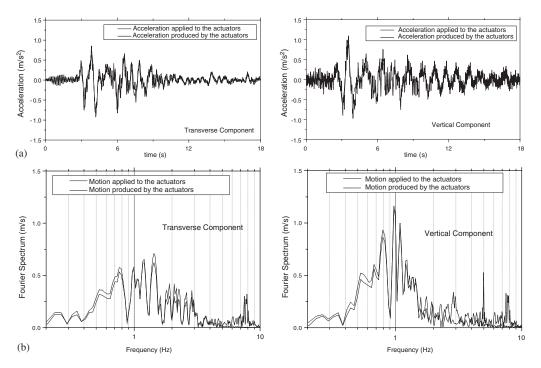
Figure 3. Comparison between the motion applied to the actuators and the motion produced by the actuators of the driving simulator. The JMA Kobe record scaled to  $PGA = 2 \text{ m/s}^2$  was used as ground motion: (a) acceleration time histories; and (b) fourier spectra.
