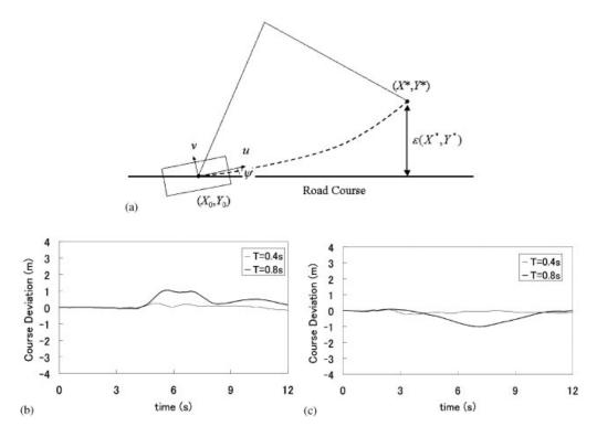
Figure 13. (a) Outline of the second-order predictable correction model; and the calculated running trajectories of the vehicle subjected to; (b) the JMA Kobe record; and (c) the El Centro record, scaled to  $PGA = 4 \text{ m/s}^2$ .
