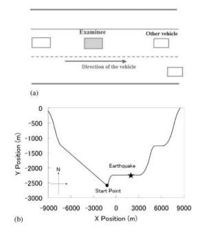
Figure 5. (a) Driving condition in the experiment; and (b) the scenario highway course programmed into the driving simulator.
