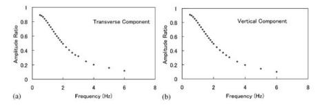
Figure 2. Amplitude ratio between the applied harmonic wave and the motion produced by the actuators: (a) transverse component; and (b) vertical component.
