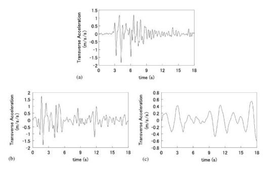
Figure 4. Absolute response acceleration time histories to the transverse direction of a running vehicle under seismic motion. The JMA Kobe and the El Centro records were scaled to  $PGA = 4 \text{ m/s}^2$ , and the SCT Mexico record was scaled to  $PGA = 1 \text{ m/s}^2$ : (a) JMA Kobe; (b) El Centro; and (c) SCT Mexico.
