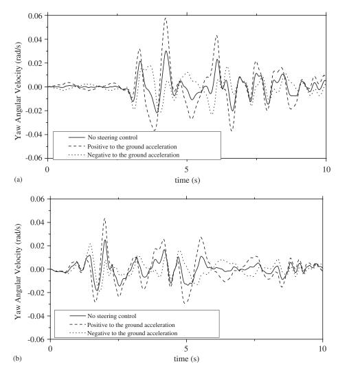
Figure 11. Comparison of the yaw angular velocities for the cases with different steering angular accelerations: (a) the JMA Kobe; and (b) the El Centro records were scaled to  $PGA = 4 \text{ m/s}^2$ .
