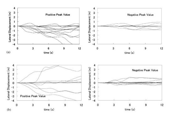
Figure 12. Running trajectory of the vehicle without considering driver's reactions (bold line) and those of the examinees (thin lines) under: (a) the JMA Kobe; and (b) the El Centro records scaled to  $PGA = 4 \text{ m/s}^2$ .
