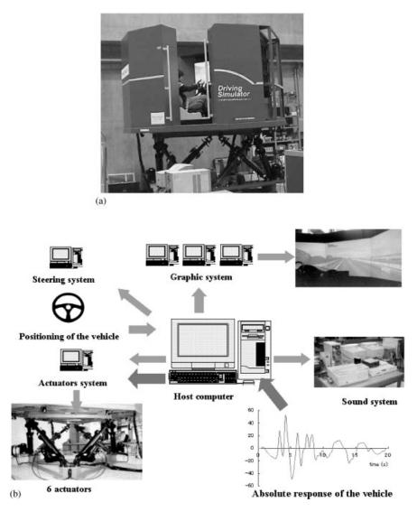
Figure 1. (a) Overview of the driving simulator used in this study; and (b) its system configuration.
