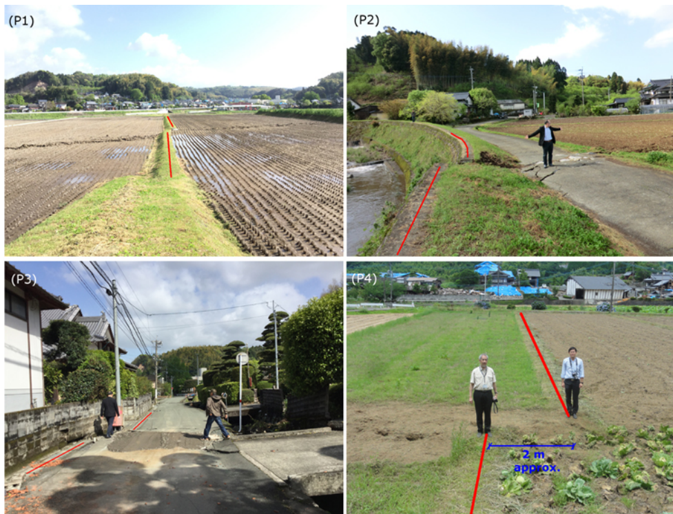
Figure 3. Examples of surface ruptures caused by the 2016 Kumamoto earthquake. Paddy field (P1), river channel (P2), road crossing in Kamijin and Shimojin districts of the town of Mashiki observed on 17 April 2016 (P3), and crop field in Dozono district of the town of Mashiki observed on 7 June 2016 (P4). The locations of the photographs are shown in Fig. 1.
