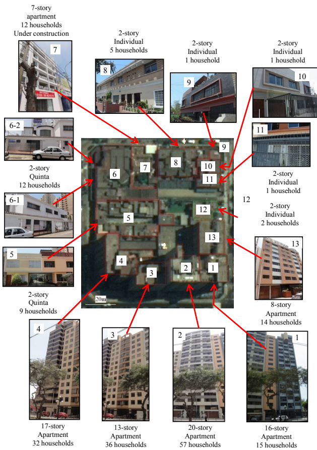
Fig. 9. Satellite image and photographs taken in the field survey for building inventory development in Lima [14].
