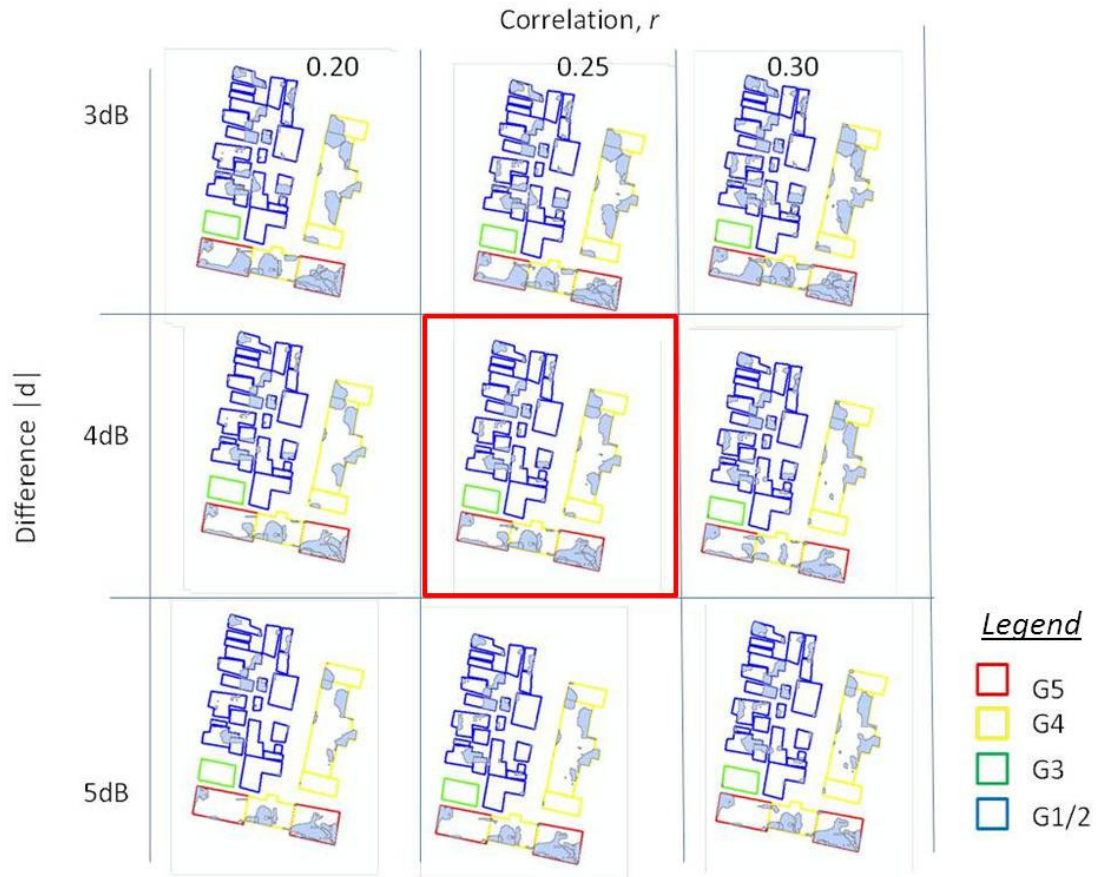
Fig.7 Example of selection of thresholds by a trial and error method for r and d in low- and moderate- density settings. Best threshold values obtained were either r \geq 0.25 or |d| \geq 4 dB and this is indicated in the central figure with red square.
