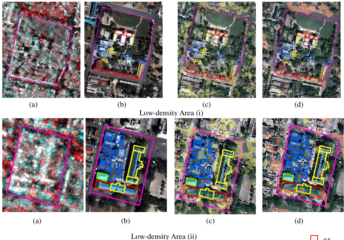
Fig. 10 Examples of low-density areas (Sample areas (i) and (ii) in Fig. 4(a)). (a) Color composite (Red: post-event scene, Cyan: pre-event scene), (b) Pre-event QuickBird image, (c) Post-event GeoEye image and subsequent overlay of low correlation, r \leq 0.25 and low NDVI ( \leq 0.3 ), (d) Overlay of high backscatter difference |d| \geq 4 dB: yellow color shows high negative d while orange color shows high positive d .
