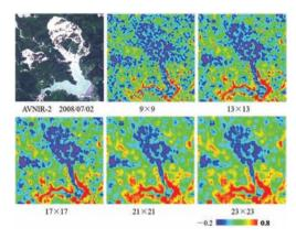
Fig. 6 Comparison of the window size for PALSAR to obtain the correlation coefficient.
