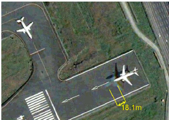
Fig. 1. Pan-sharpened QuickBird image of Ninoy Aquino International Airport in Metro Manila, Philippines, from Google Earth. A ghost is observed in front of the airplane that is landing.
