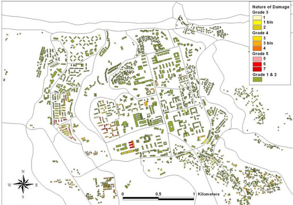
Fig. 13. Damage distribution for buildings in Boumerdes city following the 2003 Algeria earthquake. Details for each class are presented in Table 2 according to the nature of damage.
