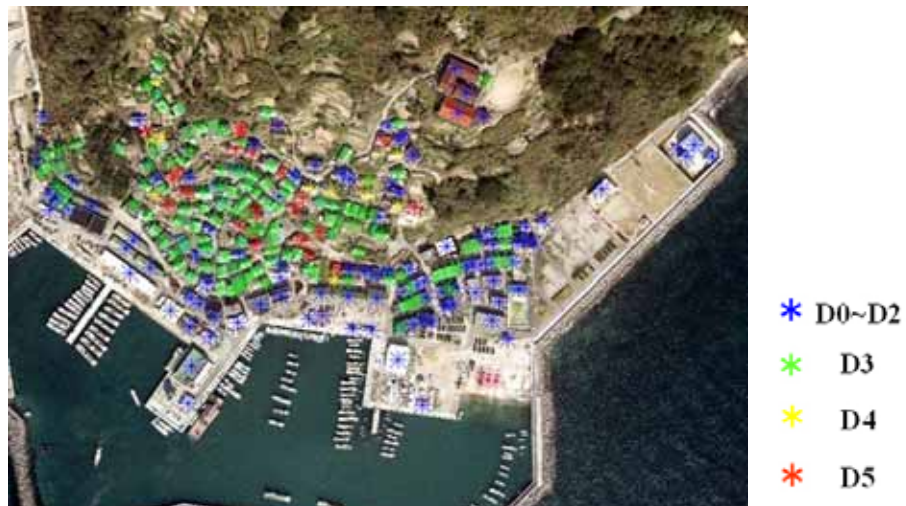
Fig. 3 Result of visual damage inspection of Genkai-jima island using a vertical aerial photograph
