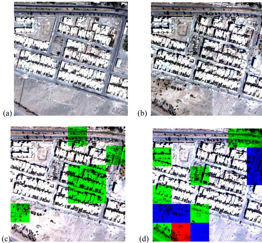
Figure 2. (a) Pre-earthquake and (b) post-earthquake image within southwestern Bam, and Damage Intensity results from (c) Maximum-likelihood classification and (d) change detection.
