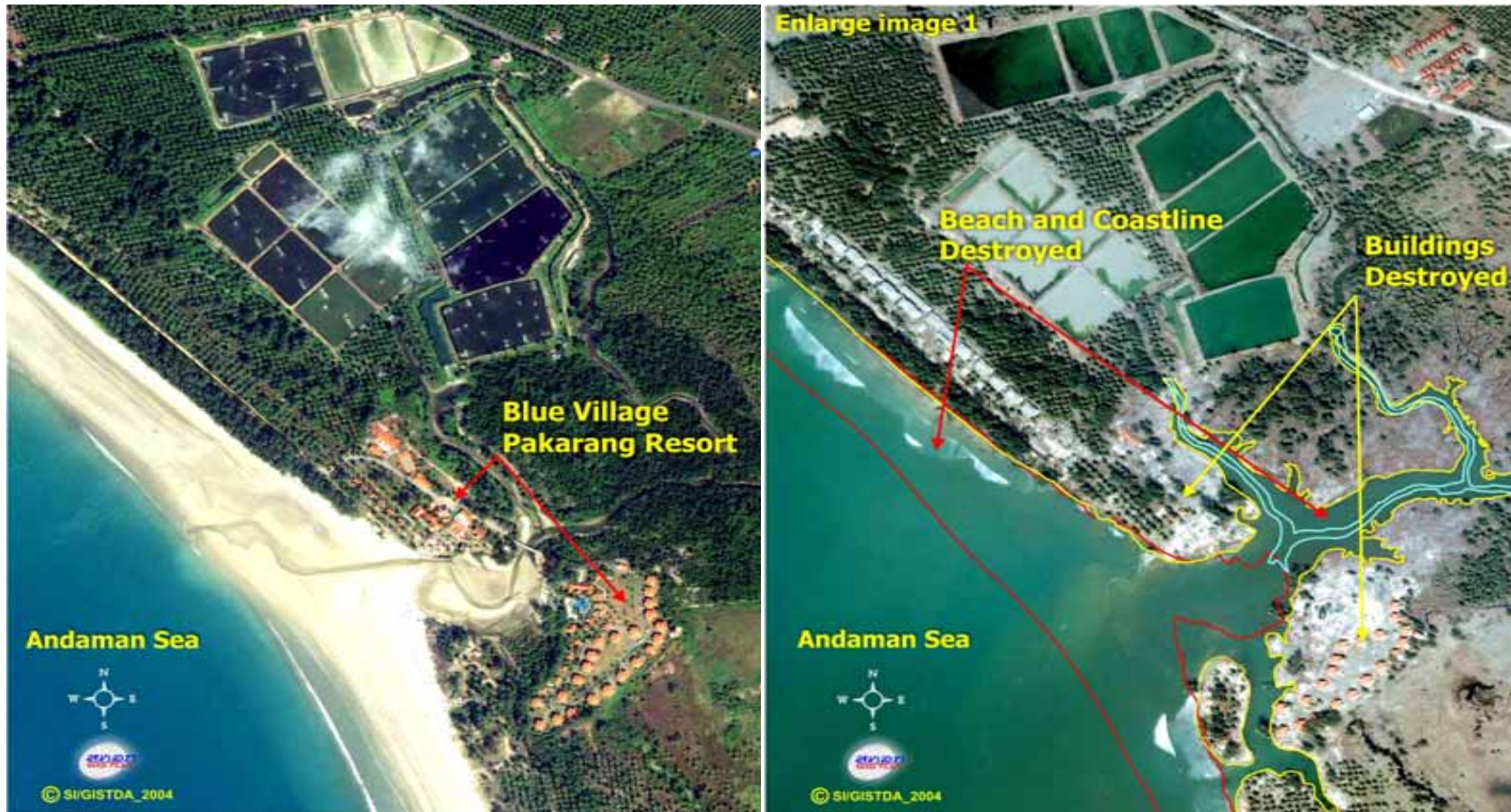
Figure 8 Pre and Post IKONOS images of the Resort, Phang-nga province acquired on January 30, 2003 (Left) and December 29, 2004 (Right) showing before and after shoreline, river bank erosion in red and yellow respectively, damages also to buildings, roads, bridges, and aquacultural farms.
