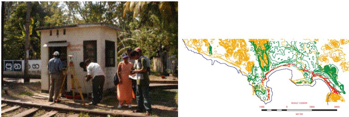
(a) Inundation measurement by the Survey Department and Coastal Conservation Department Teams (b) Different data sources used in the creation of DEM for GALLE (high elevations - existing 1:5000 data, low elevations 2ft - contour local data, coastal area - Total Station measurements)
