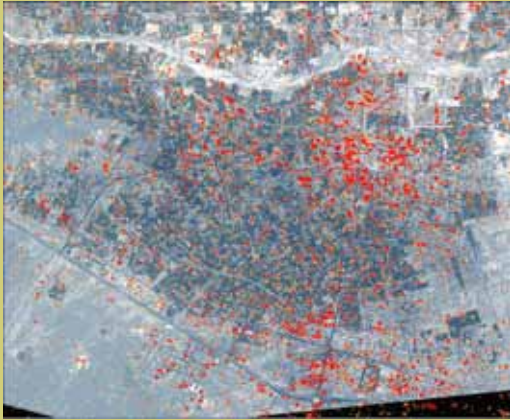
Difference in cross-powers displayed from yellow (low) to red (high) (color sliced by standard deviation differences)
